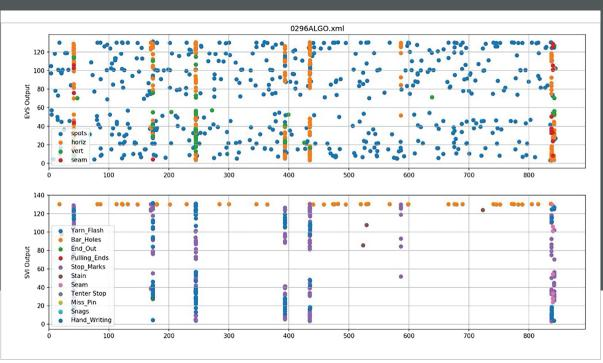
The top map plots all of the "defects" identified by the existing machine vision system on a half-mile-long fabric roll. The bottom map plots the actual defects as seen by SVI. Also note that SVI is aware of far more defect types than the machine vision system on its own.
